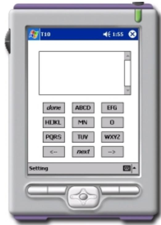
Figure 3. Constrained keypad design testing interface
